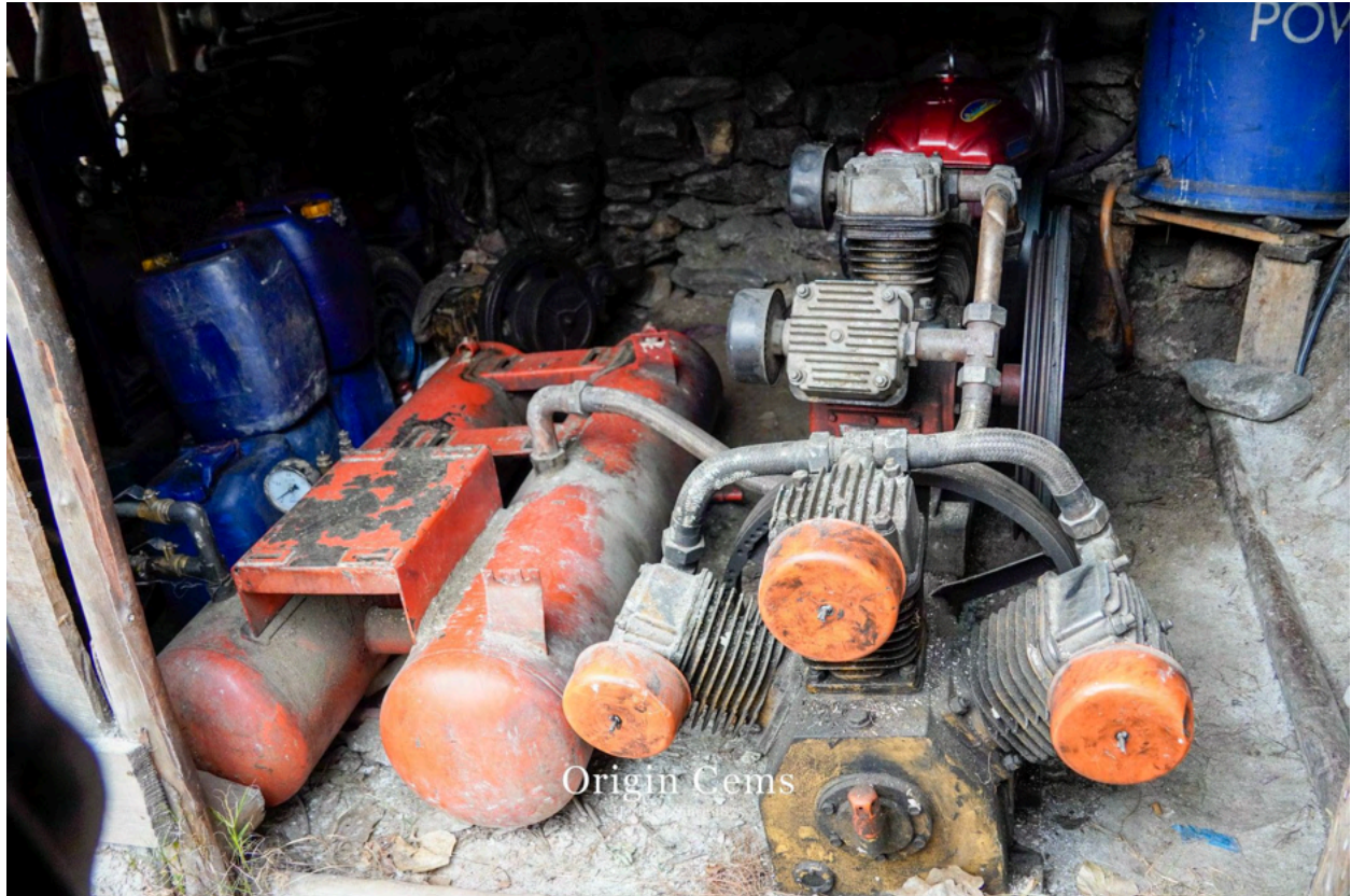
Figure 45. All over Pakistan, you will see similar compressors for the jackhammers that are used to break through the host rock in search of gemstones, in this case, Emeralds at the Gujar Killi deposit. Origin Gems® Photo.
