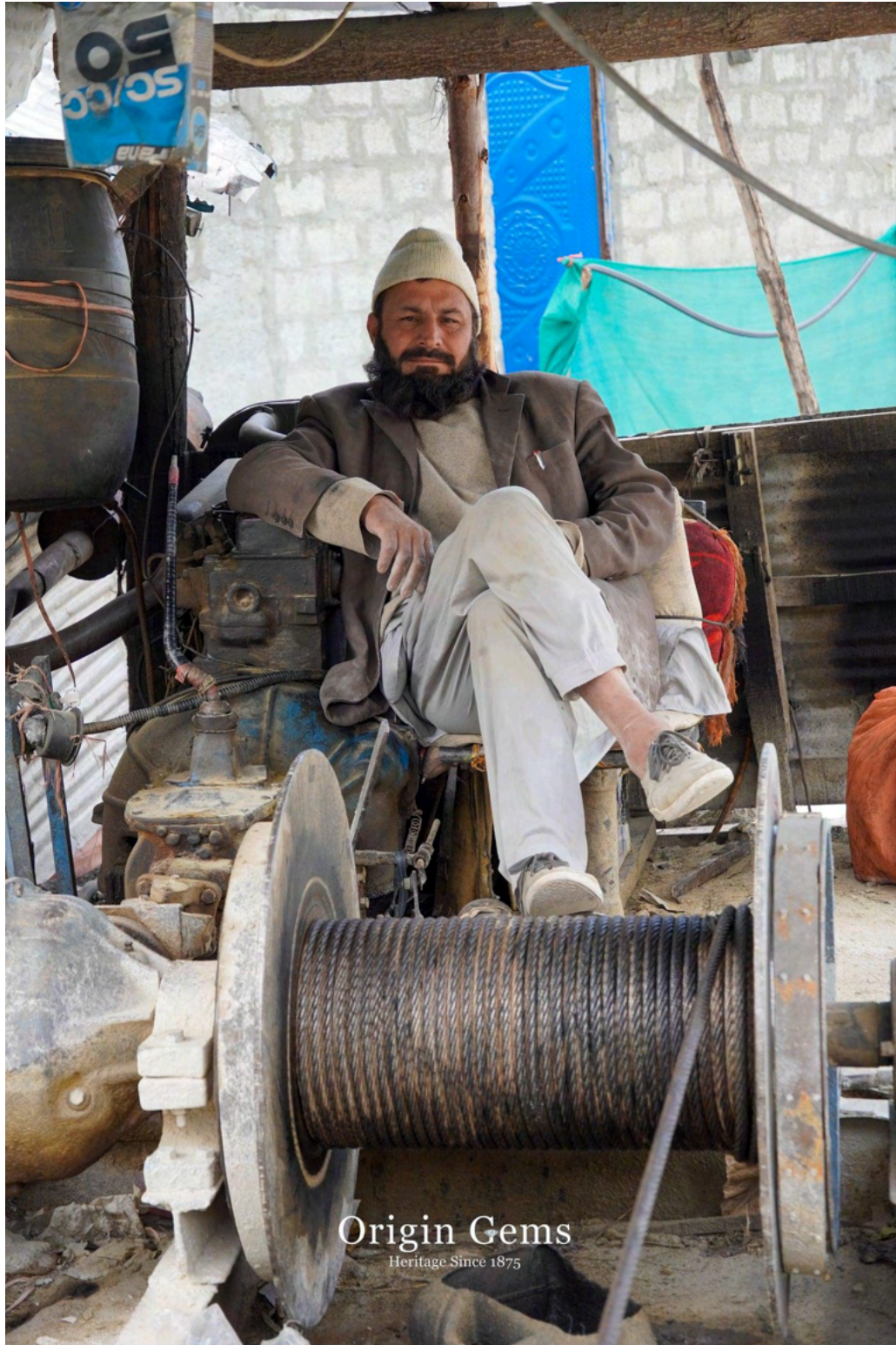
Figure 11. A controller of the pully system, a bell signals when the miners are ready to send material up or come up themselves. Origin Gems® Photo.
