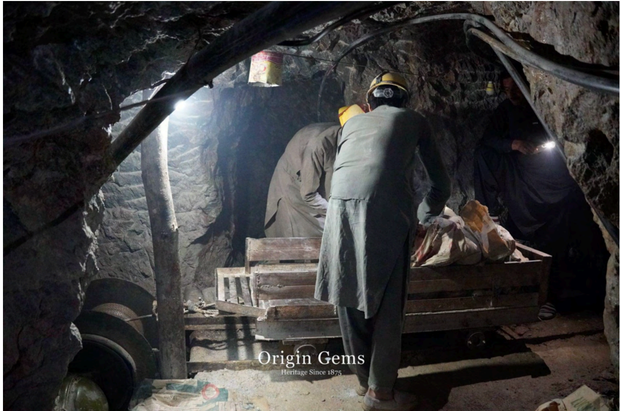
Figure 12. A pulley system inside one of the Emerald mines in Mingora, the ore is being cleared from the cart, so our team can go deeper into the mine. Before sitting, the owner of this mine's lease told us that we are responsible if anything happens in terms of safety. Mining emeralds in this environment is risky, especially as the host rock is softer and usually saturated with water. Origin Gems® Photo.
