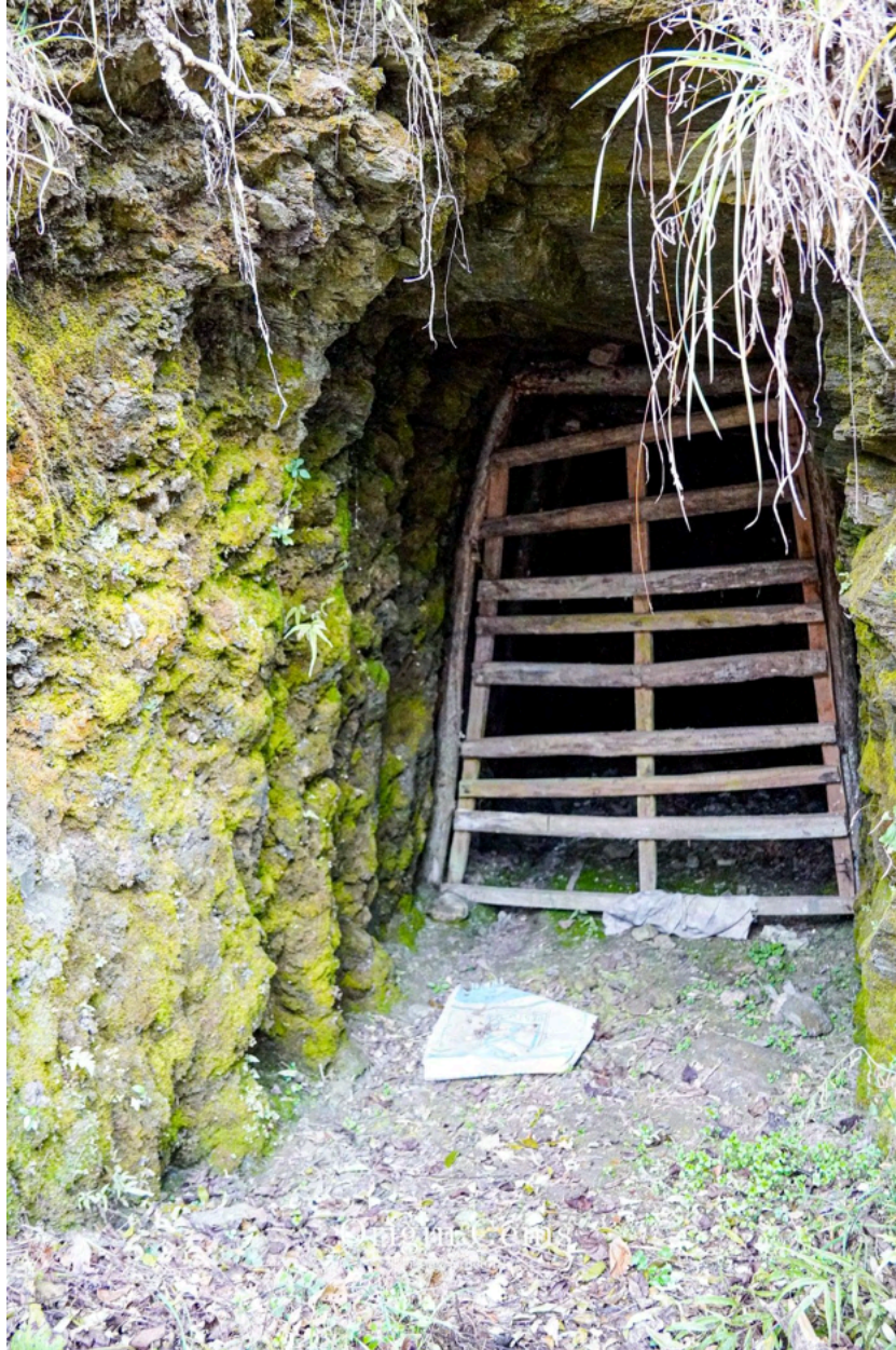
Figure 38. This mine has been closed for some time; the miners didn't find feasible production in this tunnel, so they had to close and resume operations from a different angle, going deeper in the deposit. Taken in December 2024 at the Gujar Killi (Amni) Emerald deposit site. Origin Gems® Photo.
