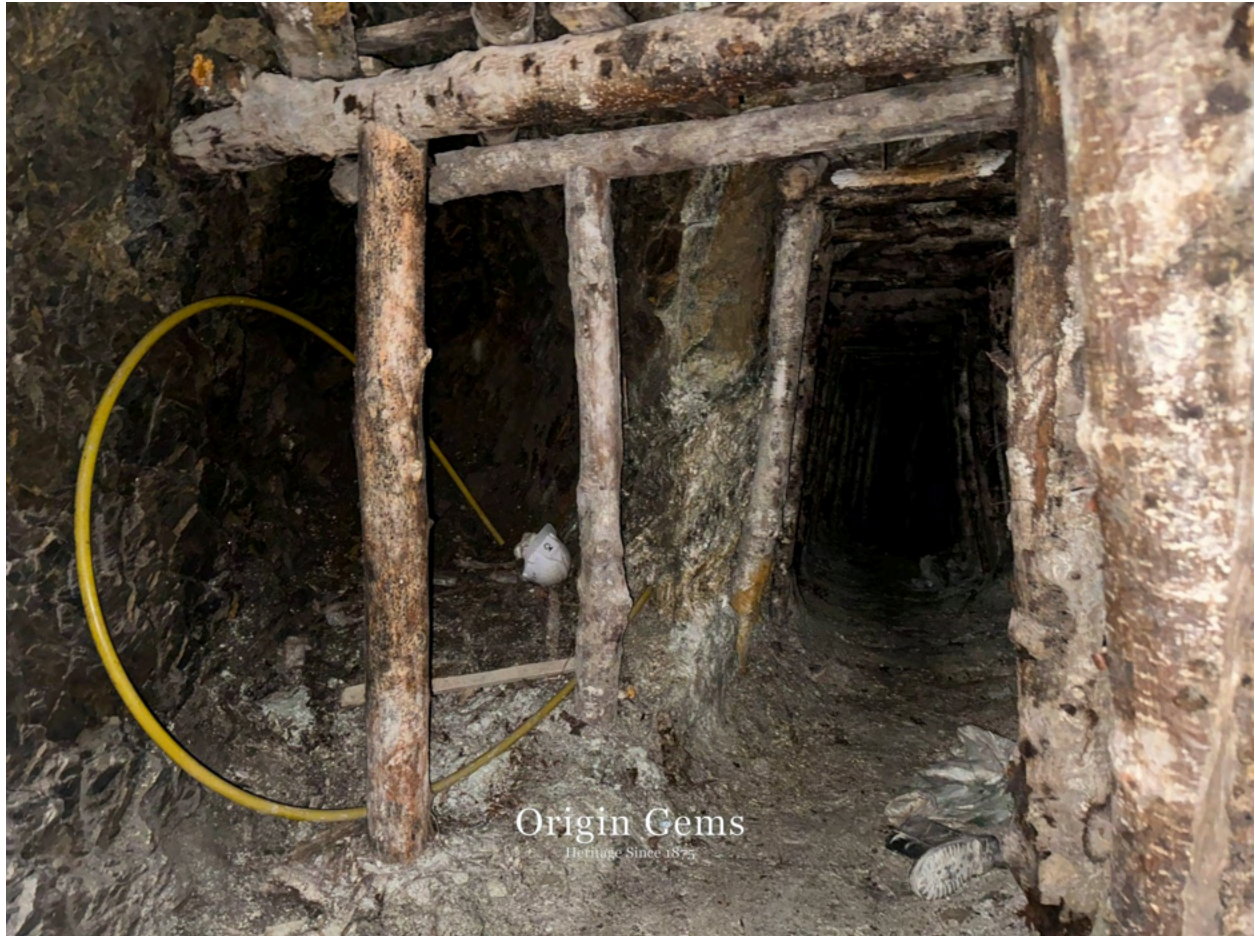
Figure 42. Inside the Gujar Killi Emerald mine tunnels, held up by wood. Origin Gems® Photo.
